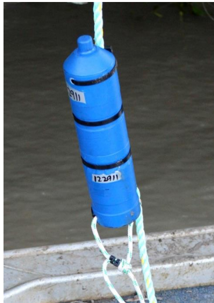
Figure 11. An example of an acoustic receiver (VEMCO VR2W), which has been coated with antifouling paint for an estuarine deployment.
