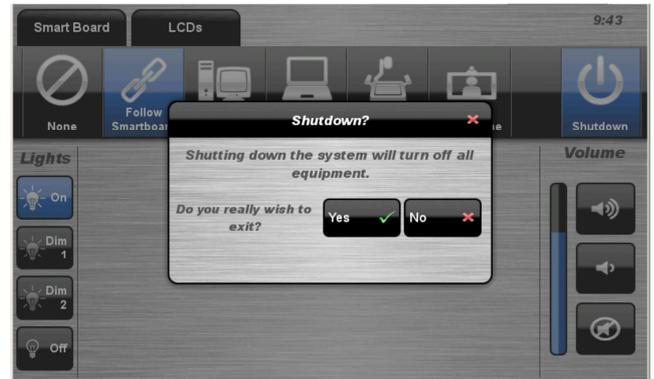
**NOTE:** Letting the system go to sleep by itself only powers down the touch panel screen, it does not turn off the audio-visual equipment. To turn off the equipment, shutdown the system properly using the touch screen panel. This will extend the life of the audio-visual equipment
