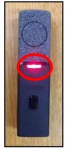
**To turn on** -> Remove from charging dock and wait for 3 seconds, until the LED flashes red. Press button on mic to activate. The LED lights will flash green every few seconds to show that the microphones are active.
